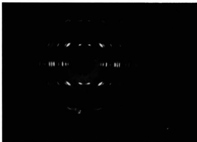
Fig. 1. L-Tyrosine. Fibre pattern about the [001] axis, Cu K\alpha radiation; camera radius = 3 cm.
